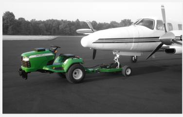
Attaches to tire only. Protects limited caster aircraft by patented design of attaching and holding
