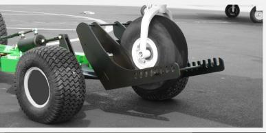
Dual wheel lift system will lift up to 12", lowering the tail for low door headers.
